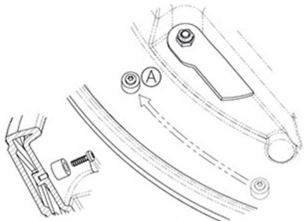
The figure on the right shows the child protection lock in an inspection shaft in the closed position.
