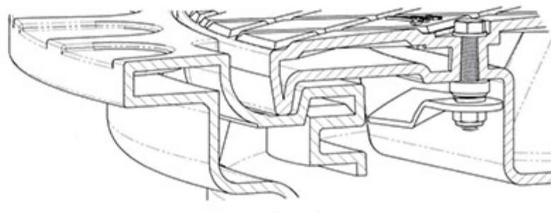
The locking bolt (A) prevents the cover spinning. It must be fixed in the correct position in the shaft extension or the inspection shaft of the tank.
