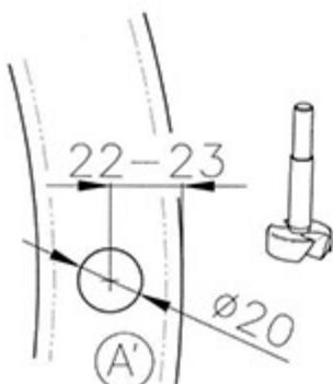
With inspection shaft directly on the tank, the drilled hole for the locking bolt is aligned to the cover. If this needs adjusting, an additional drilling of A' can be made, see figure on the left.
