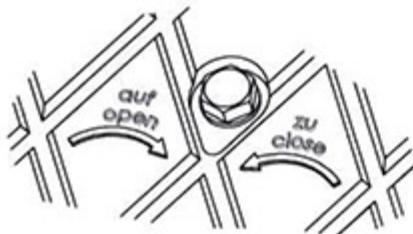
By turning the hexagonal screw on the upper side of the cover, the bolt (B) is operational and the child protection bolt is closed. The bolt slides into a pocket or grips the inner edge of an inspection shaft. (Point 2.2.1) Maximum one quarter rotation is necessary. The rotation direction is given on the top of the cover.
