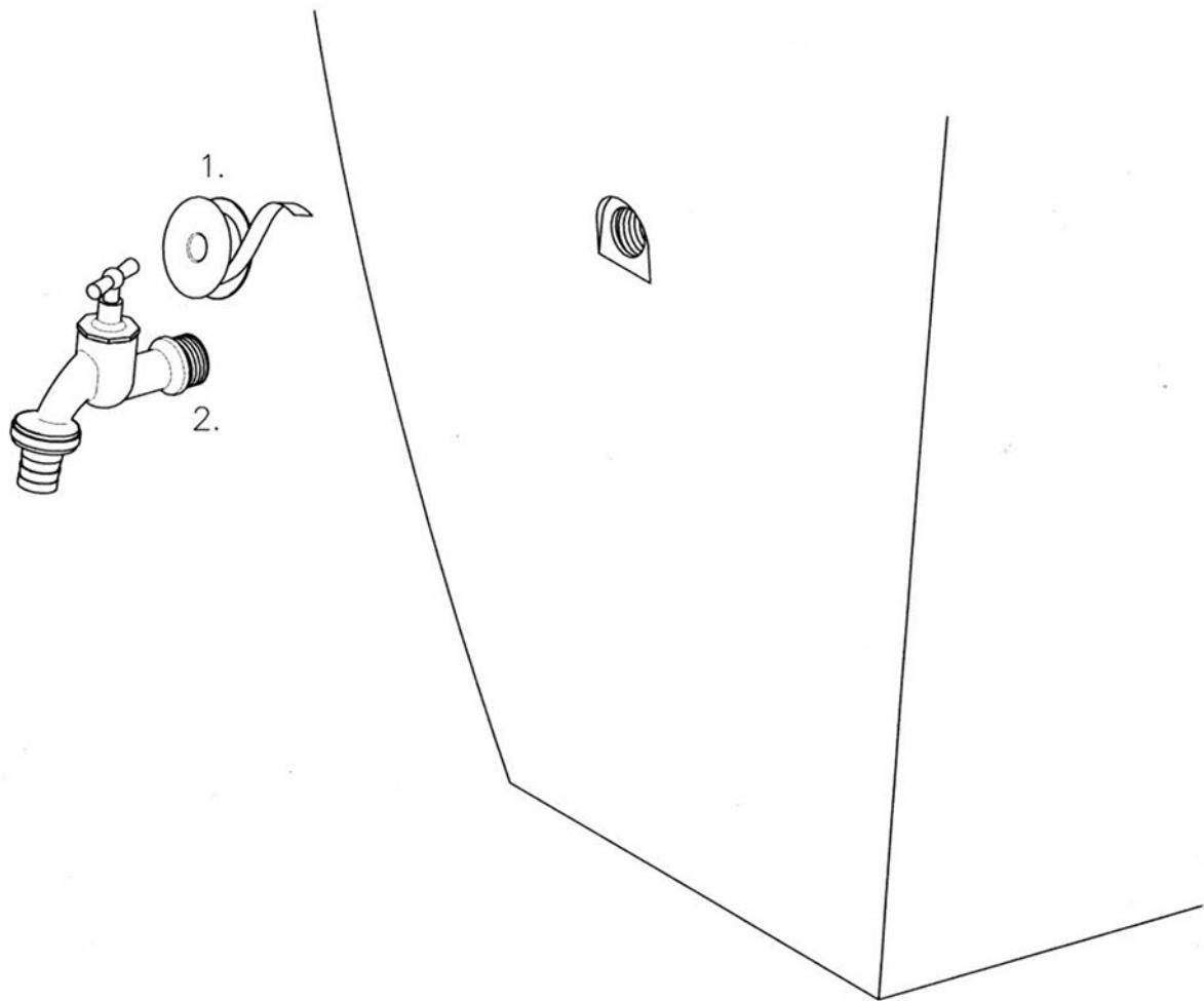
**1.** Apply a sealant to the thread of the tap.
